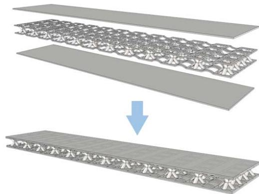
Figure 5. Plastic sandwich panel with pyramidal kagome core
