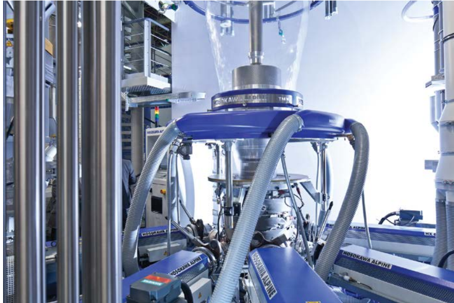
Figure 2. A traditional 5-layer coextrusion blown film line showing a nested spiral die, air ring and bubble. Courtesy Alpine American.
