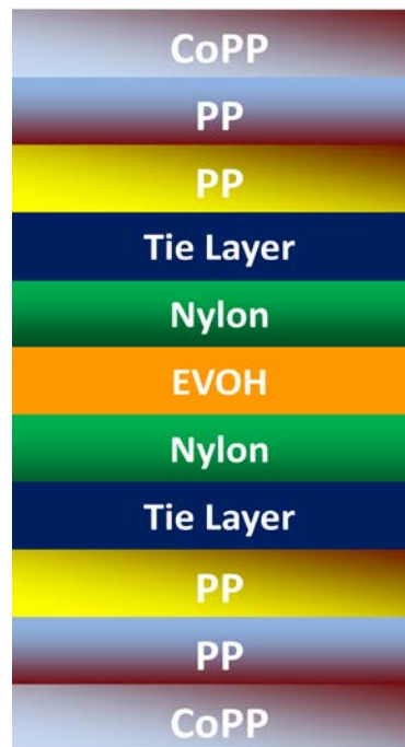
Fig. 3E 11-layer retortable, high-barrier structure using cost/performance optimized PP and copolymer PP resins
