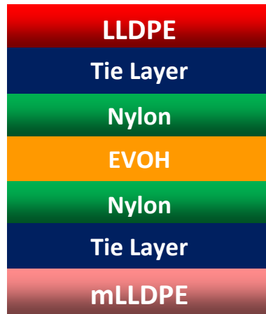
Fig. 3B High barrier lidding structure
