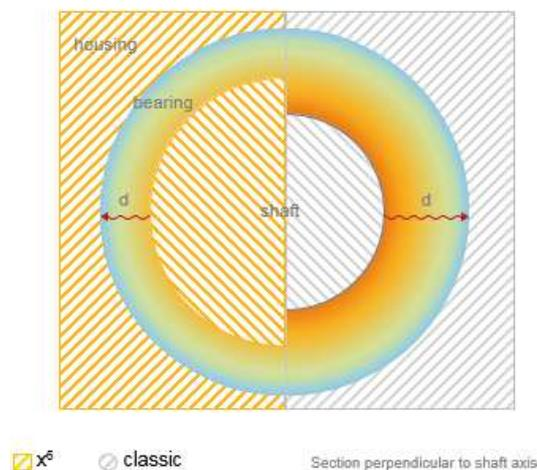
Figure 2: Modified bearing design reduces bearing temperature and effectively increases the pump speed limit to make higher flow rates possible.
