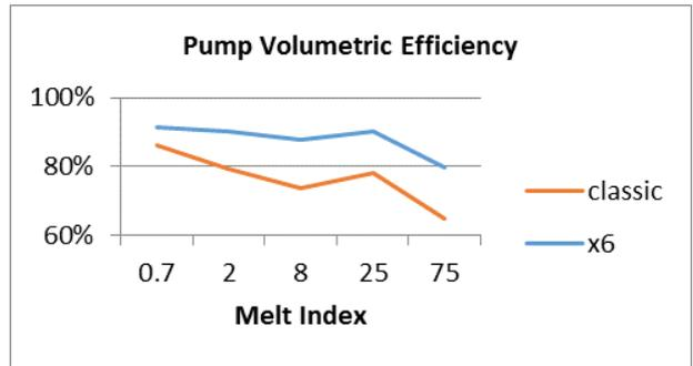
Figure 8: In the 20 tph PP plant, a classic pump operates at 76% volumetric efficiency, while the x6 class pump operates at 88% volumetric efficiency.
