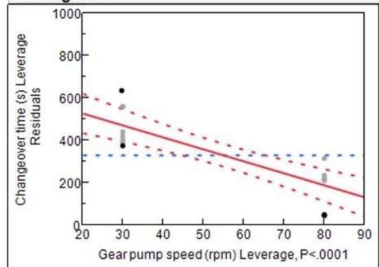
Figure A. Model fit for SSE changeover time, as a function of viscosity ratio and gear pump speed
