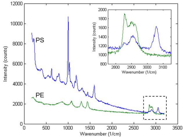
Figure 1. Raman spectra of pure PE and PS
