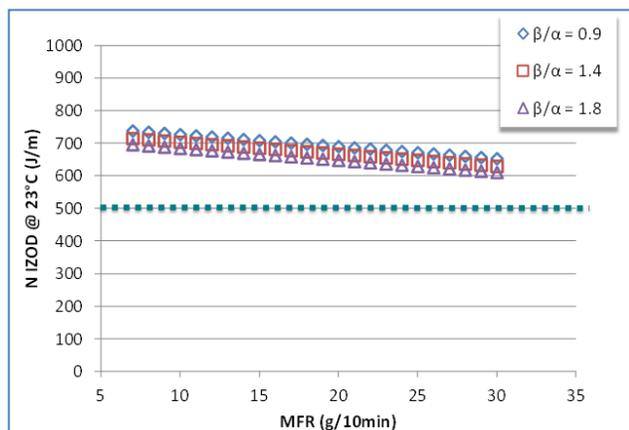
Figure 7: Room temperature izod as a function of MFR for modeled r-TPO's (empirical correlations done on 6<sup>th</sup> generation based TPO's).  $EPR^c$  is 33 w% for all modeled systems in the graph.
