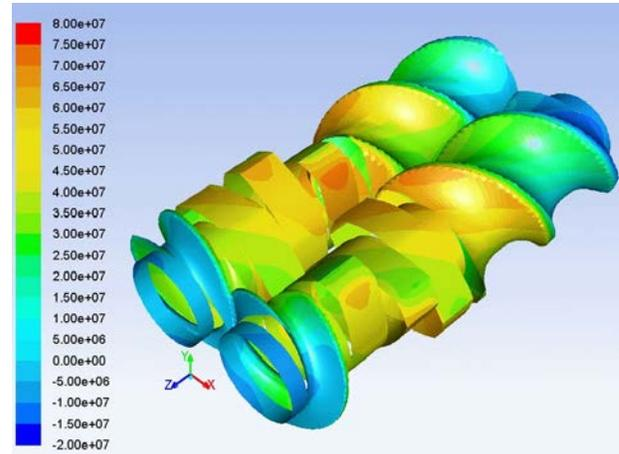
Figure 4: FEM simulation of screw element sequence
