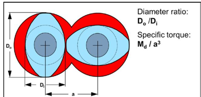
Figure 1: Character dimensions of Twin-screw Extruder
