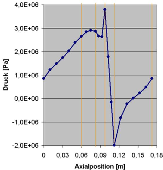
Figure 6: Pressure drop value across restrictive elements
