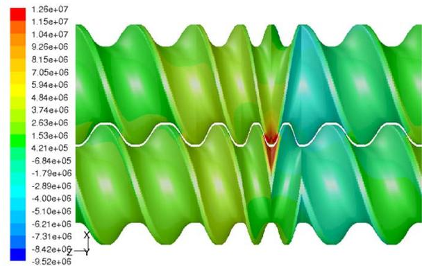
Figure 7: Pressure drop details at restrictive element.
