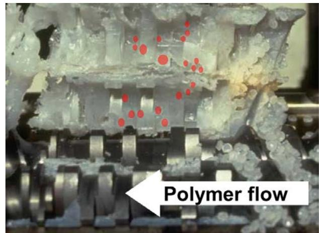
Figure 11: Melting zone showing transformation of polymer
