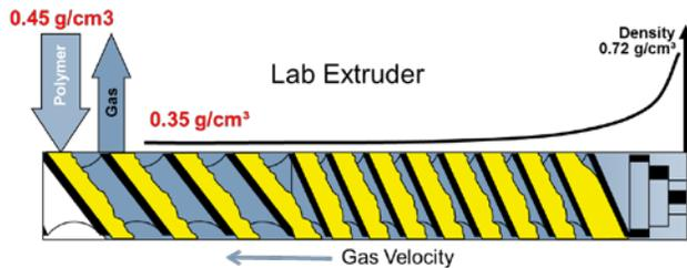
Figure 9: Powder feedstock conveying in lab compounder.
