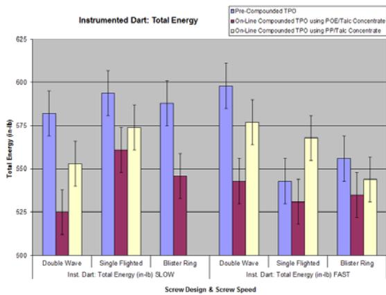
Figure 9: TPO Sheet – Instrumented Dart Impact.
