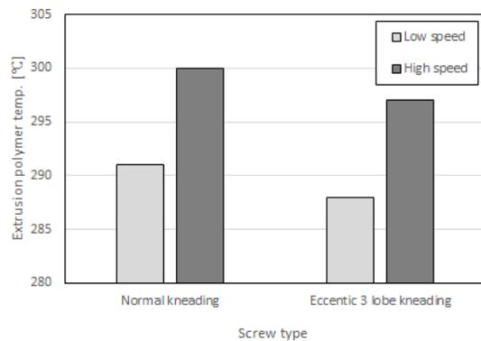
Chart 3: Relationship between screw configuration and polymer temperature.
