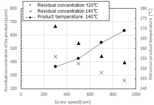
**Chart 1: Relationship between screw rpm and residual concentration of by-products**
