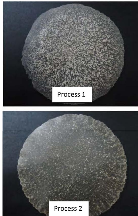
Photo 4 Fiber dispersion on each mixing processes
