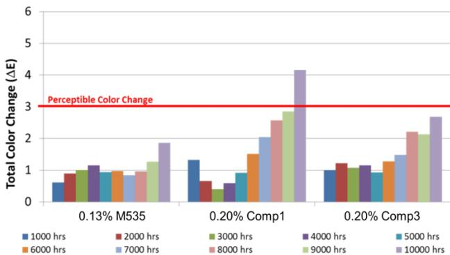
Figure 3 | Total color change in natural HDPE after 10k hours G155 weathering. Samples contain CYANOX<sup>®</sup> 2777 antioxidant.
