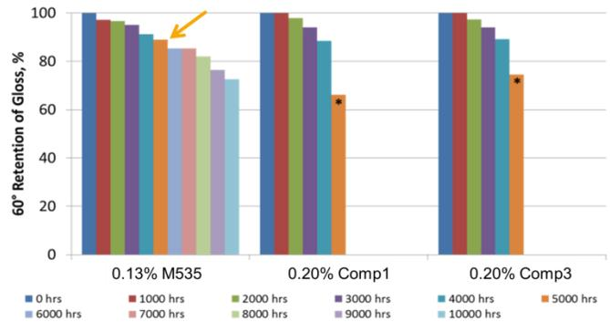
Figure 5 | 60° retention of gloss in green HDPE after 10k hours G155 weathering. The (\*) denotes surface crazing.
