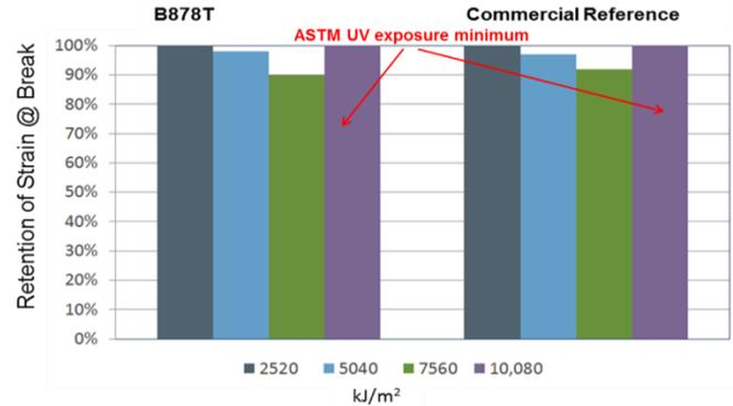
Figure 8 | TPO roofing sheet – retention of strain at break after 10,080 kJ/(m<sup>2</sup>·nm) radiant energy in an ASTM D6878 weatherometer
