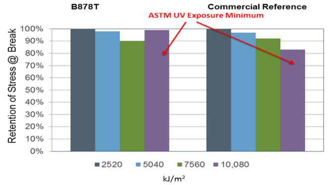
Figure 7 | TPO roofing sheet – retention of stress at break after 10,080 kJ/(m<sup>2</sup>·nm) radiant energy in an ASTM D6878 weatherometer
