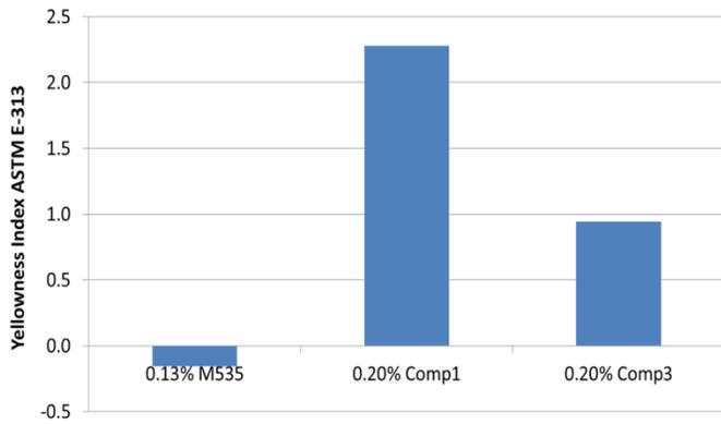
Figure 2 | Initial color of HDPE containing various stabilizers and CYANOX<sup>®</sup> 2777
