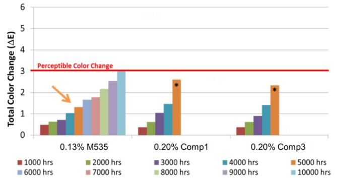
Figure 4 | Total color change in green HDPE after 10k hours G155 weathering. The (\*) denotes surface crazing.
