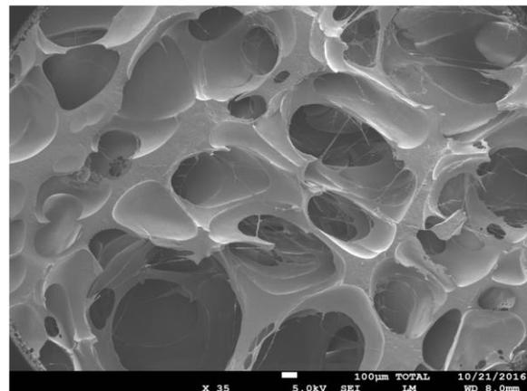
Figure 5. SEM image of conventional PP processed with 0.6mL/min CO<sub>2</sub> at 130 bar die pressure
