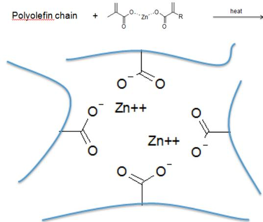
Figure 1. Reaction of zinc salts with polyolefin chain.
