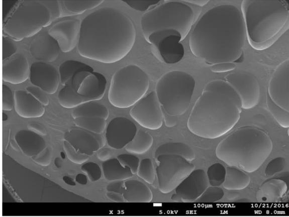
Figure 6. SEM image of conventional PP modified with 1% Dymalink® 9200 processed with 0.6mL/min CO<sub>2</sub> at 130 bar die pressure
