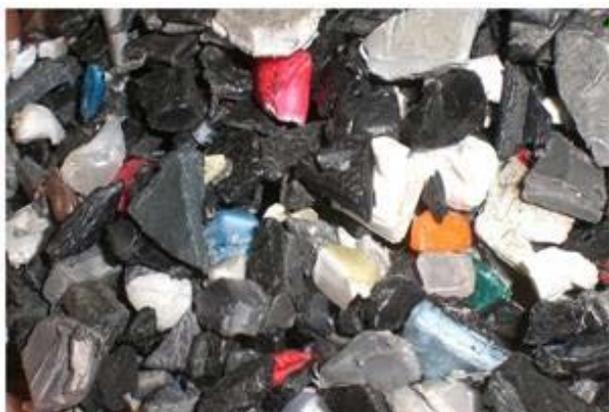
Figure 3. PP flakes recovered from upgraded ASR
