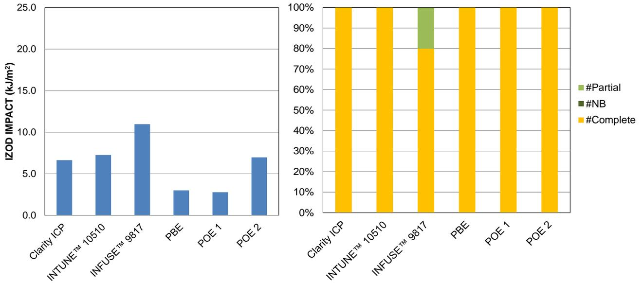
Figure 4 – Izod Impact and Failure type at -20°C
