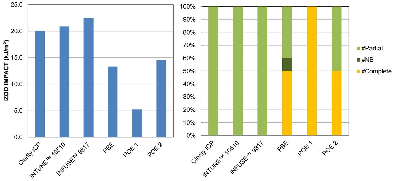
Figure 2 – Izod Impact and Failure type at 23°C
