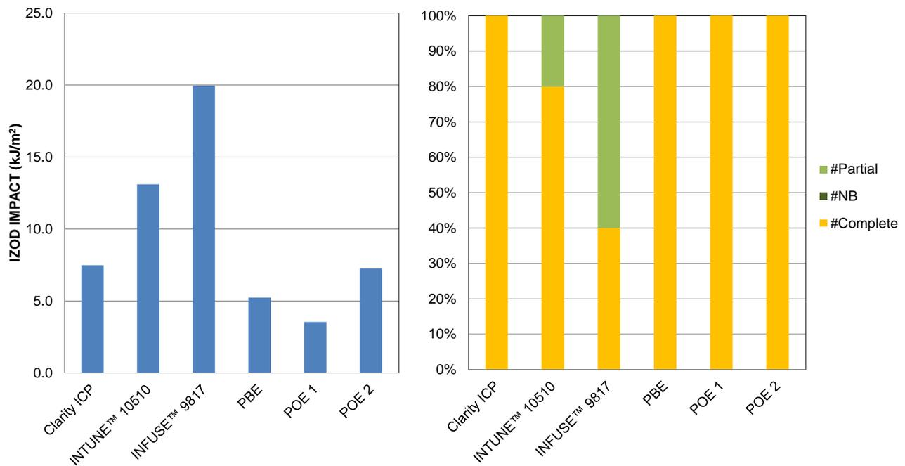
Figure 3 – Izod Impact and Failure type at 0°C
